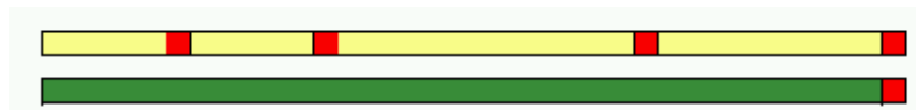
Figure 1: Cutting addition transform adds cut size to items (top) and to bin (bottom)
